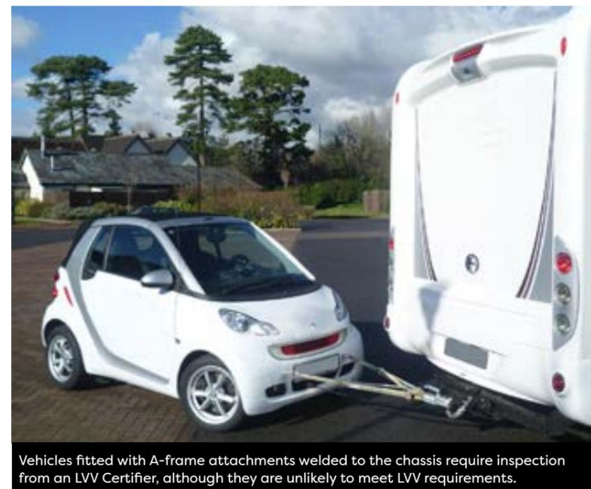
Vehicles fitted with A-frame attachments welded to the chassis require inspection from an LVV Certifier, although they are unlikely to meet LVV requirements.
