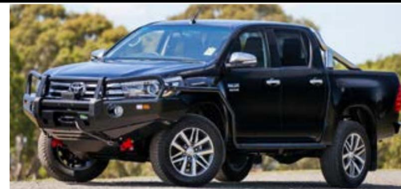
Vehicles required to meet frontal impact occupant protection standards (see breakout box on previous page), can only be fitted with frontal impact-compliant accessories. Home-made or custom auxiliary bars cannot be accepted.
