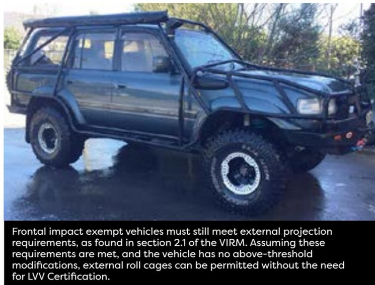
Frontal impact exempt vehicles must still meet external projection requirements, as found in section 2.1 of the VIRM. Assuming these requirements are met, and the vehicle has no above-threshold modifications, external roll cages can be permitted without the need for LVV Certification.
