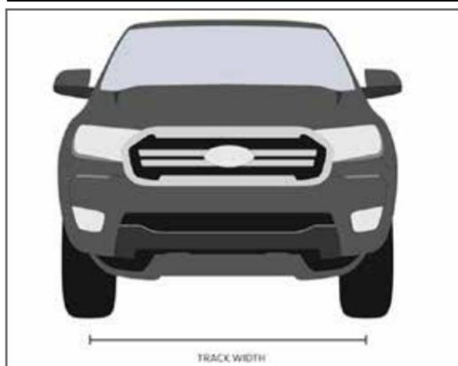
The previous wording of the VIRM threshold allowed wheel track to increase no more than 25mm in total before LVV certification was required.
