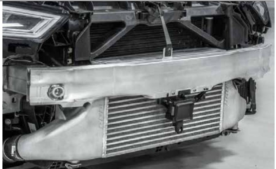
**Class MA vehicles produced after 1 March 1999 that are fitted with aftermarket intercoolers should be assessed during a Warrant of Fitness inspection to ensure that the structure of the vehicle has not been modified. Vehicles with modified structure should be referred for LVV Certification.**
