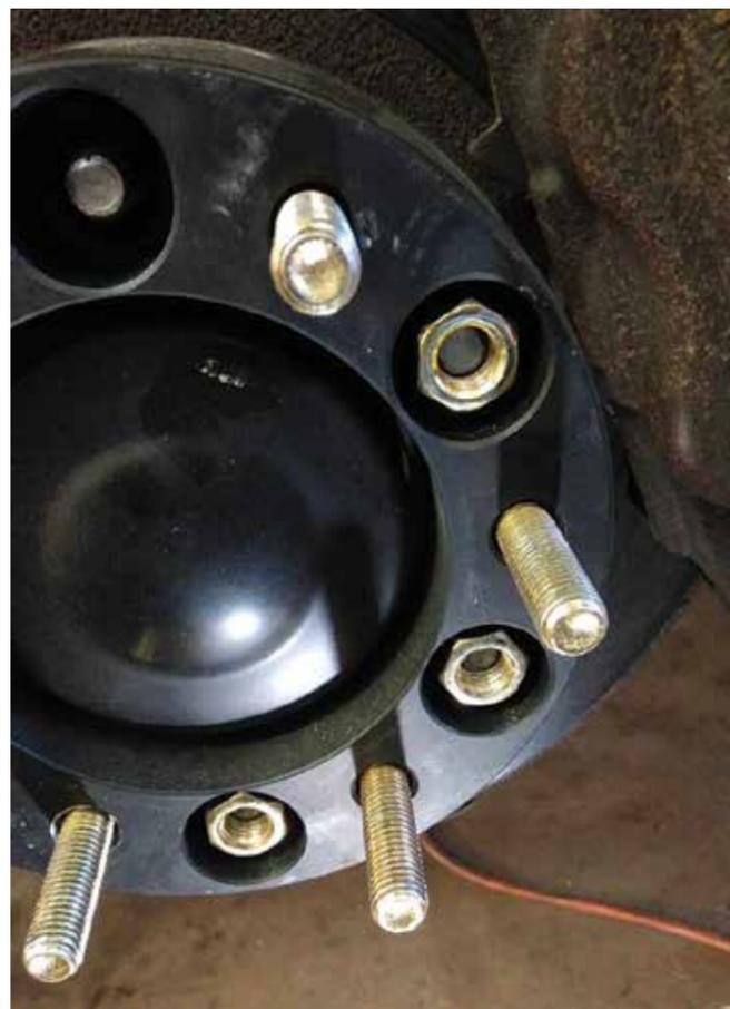
Any vehicle fitted with aftermarket wheel spacers or adaptors requires LVV Certification before a Warrant of Fitness can be issued. Part of the inspection process is to ensure thread engagement meets requirements. The example shown here has dangerously-low thread engagement.
