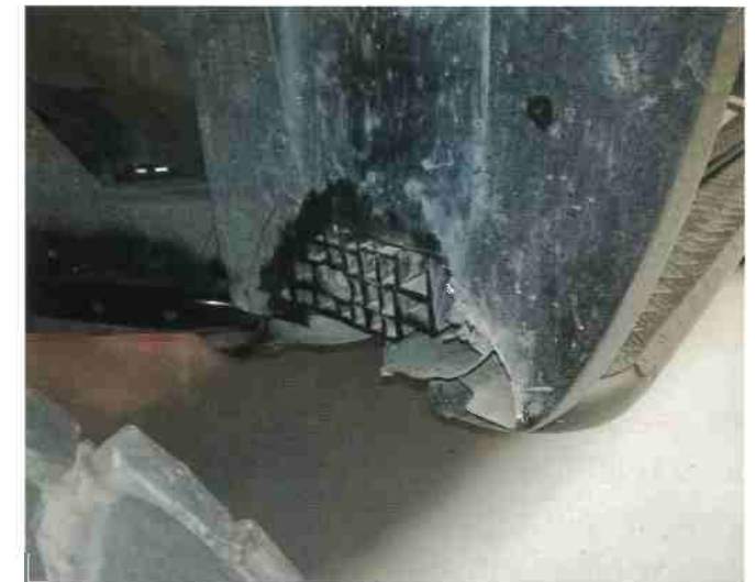
Damage to wheel arch liners can indicate the tyre size has been increased.
