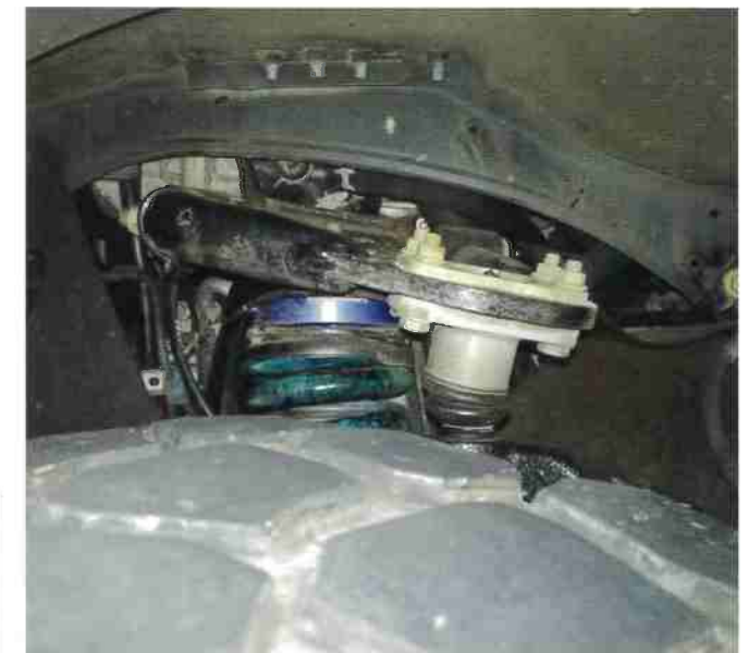
Strut spacers and extended ball joints both need to be LVV certified.
