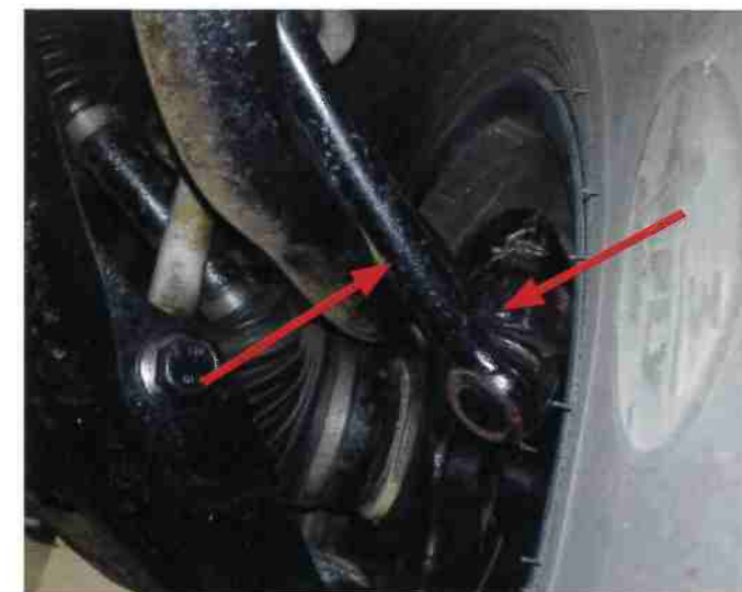
Common issues with raised suspension are binding joints and components fouling.
