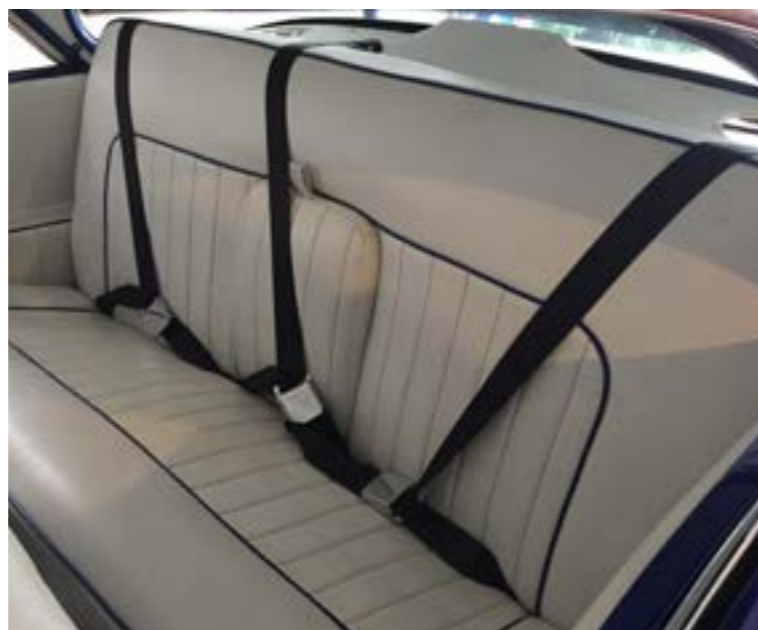
Retrofitted 3-point seatbelts, known as lap and diagonal, in the rear of a 1956 Cadillac.
