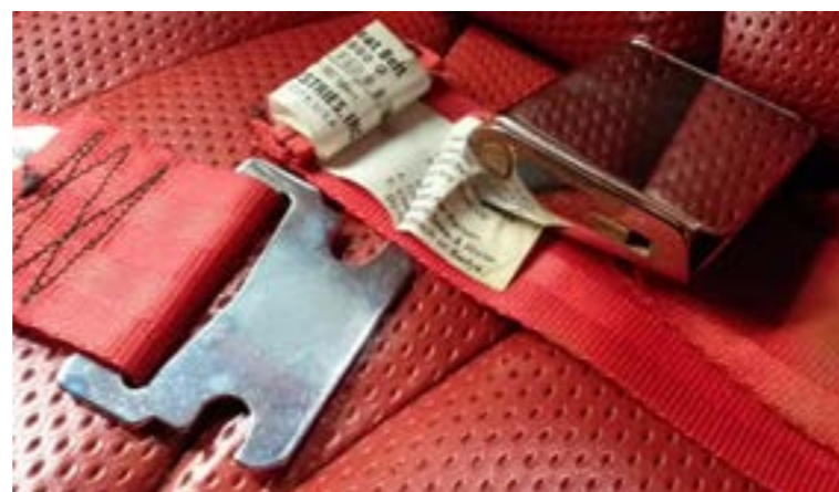
The date on this lap belt in a 1964 Cadillac is February 1993 so not original and would not meet exception 1. However, the vehicle weighs 2,200kg so 3-point static belts are not required – exception 2 is met and the lap belts are acceptable.
