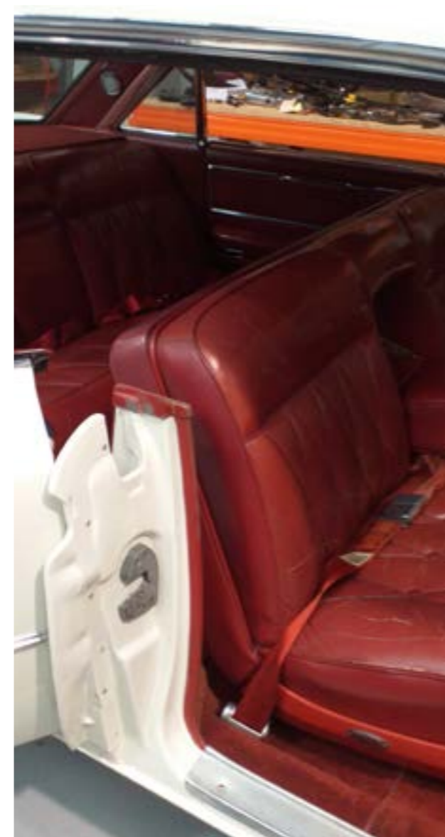
This 4-door Cadillac has a roof but without a full B-pillar there is no suitable structure in the permitted area for an upper anchorage. Lap belts are acceptable.
