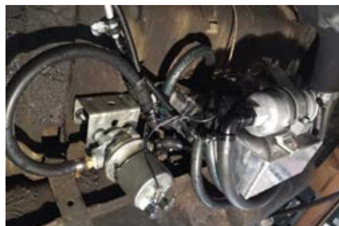
Fuel system components under rear of a 60s Chev for a fuel injected LS1 V8
