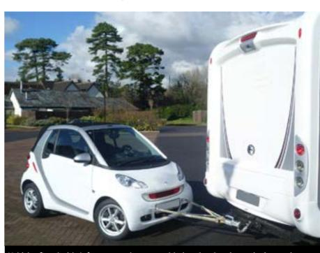
Vehicles fitted with A-frame attachments welded to the chassis require inspection from an LVV Certifier, although they are unlikely to meet LVV requirements.
