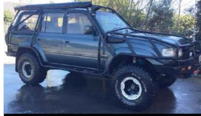
Frontal impact exempt vehicles must still meet external projection requirements, as found in section 2.1 of the VIRM. Assuming these requirements are met, and the vehicle has no above-threshold modifications, external roll cages can be permitted without the need for LVV Certification.
