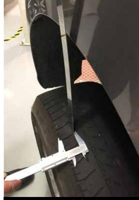
A tyre that's tread protrudes from the OE unmodified original body panels by less than 25mm, as shown here, can be accepted if covered with an aftermarket flare.
