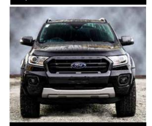
The aftermarket wheels fitted to this vehicle are covered by aftermarket fender flares, however the tyre tread does not extend by more than 25mm outside of the unmodified original body panels, and so no LVV certification is required.
