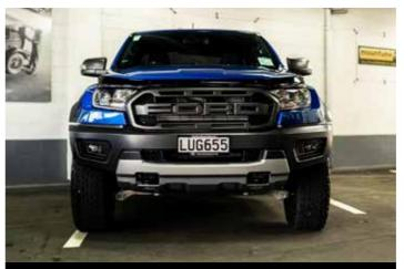
The Ford Ranger Raptor is factory-fitted with wide steel guards and plastic fender flares, the tyre tread is already 25mm outside of the unmodified original [steel] body panels, so any increase in wheel track on this vehicle would require LVV certification.
