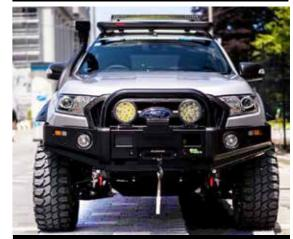
Fitted with aftermarket wheels, tyres, and mudguard extensions, this vehicle requires LVV certification due to the tyre tread extending further than 25mm outside of the unmodified original body panels, or factory-fitted mudguard extensions.
