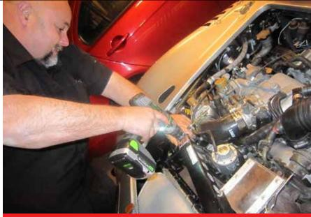
Ensure that the area behind the certification plate is clean, the backing paper is removed and that no damage is made to wiring or fuel system components when drilling the attachment holes.
