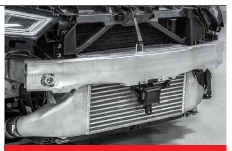
Class MA vehicles produced after 1 March 1999 that are fitted with aftermarket intercoolers should be assessed during a Warrant of Fitness inspection to ensure that the structure of the vehicle has not been modified. Vehicles with modified structure should be referred for LVV Certification.
