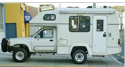
WoF inspectors are advised to keep an eye out for vehicles which may exceed their GVM and ensure that tyres are rated for the possible load carrying capacity.
