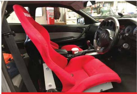
Any vehicle where the seatbelt anchorage has been changed or moved from OE requires LVV Certification. The seatbelt buckle is attached to the frame of this aftermarket seat, so this seatbelt anchorage must be LVV Certified.
