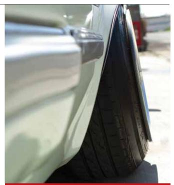
For both WoF and LVV Certification no part of the tyre tread should extend beyond the OE bodywork or aftermarket flares/mudguard extensions. Tyres must also be suitable for the wheel size.
