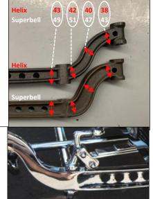
LVVTA requires LVV Certifiers certifying a vehicle fitted with a Helix axle of this design to reject the axle, and advise the vehicle owner to cease using the vehicle until the axle is replaced with a safe and compliant axle.
