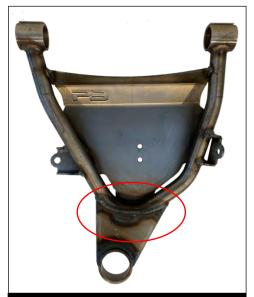
**Above:** A PBFab (Porterbuilt) Chevrolet C10 lower arm showing the cantilever-style ball joint platform design (which is the only issue that was identified with this particular arm).
