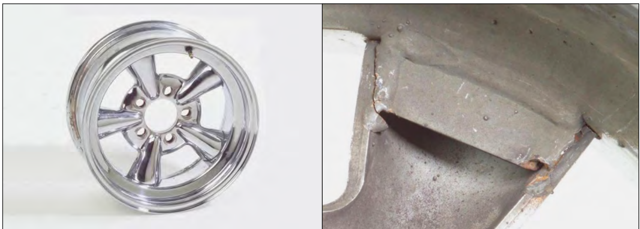
Left: Front face of typical copy of an Astro Supreme-brand wheel. Right: Weld failures on a copy of an Astro Supreme-brand wheel.
