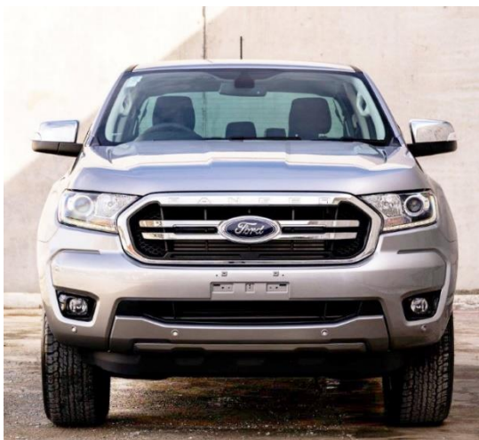
Standard vehicle - Wheels and tyres under the unmodified original guards: LVV certification is not required.
