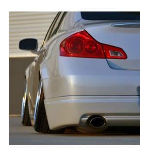
However, the effect of excessive negative camber in a normal road car application, particularly when wide low-profile tyres are fitted, can be to reduce a vehicle's grip level due to the reduction in the tyre-to-road contact patch, particularly during normal road driving in wet conditions.
