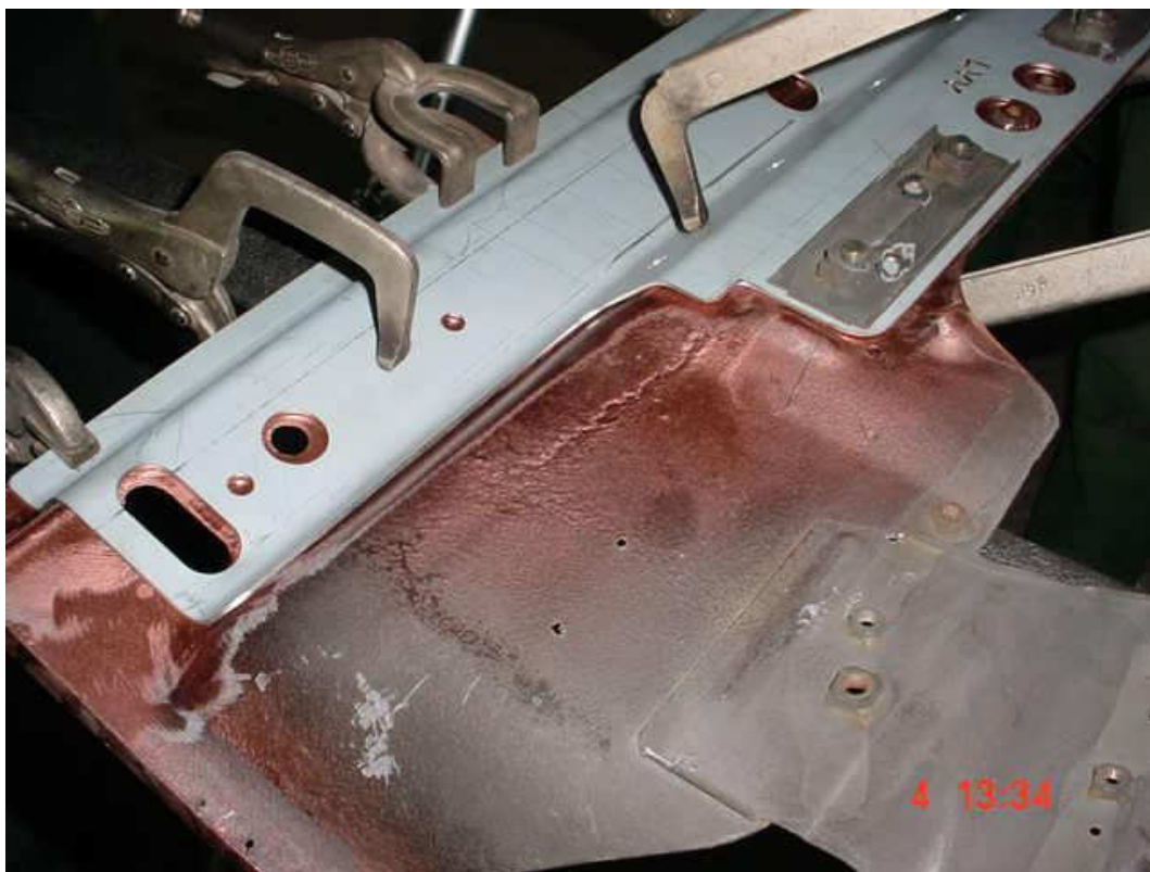
Seatbelt bolts through the seatbelt-anchorage plates help clamp the assembly for welding.
