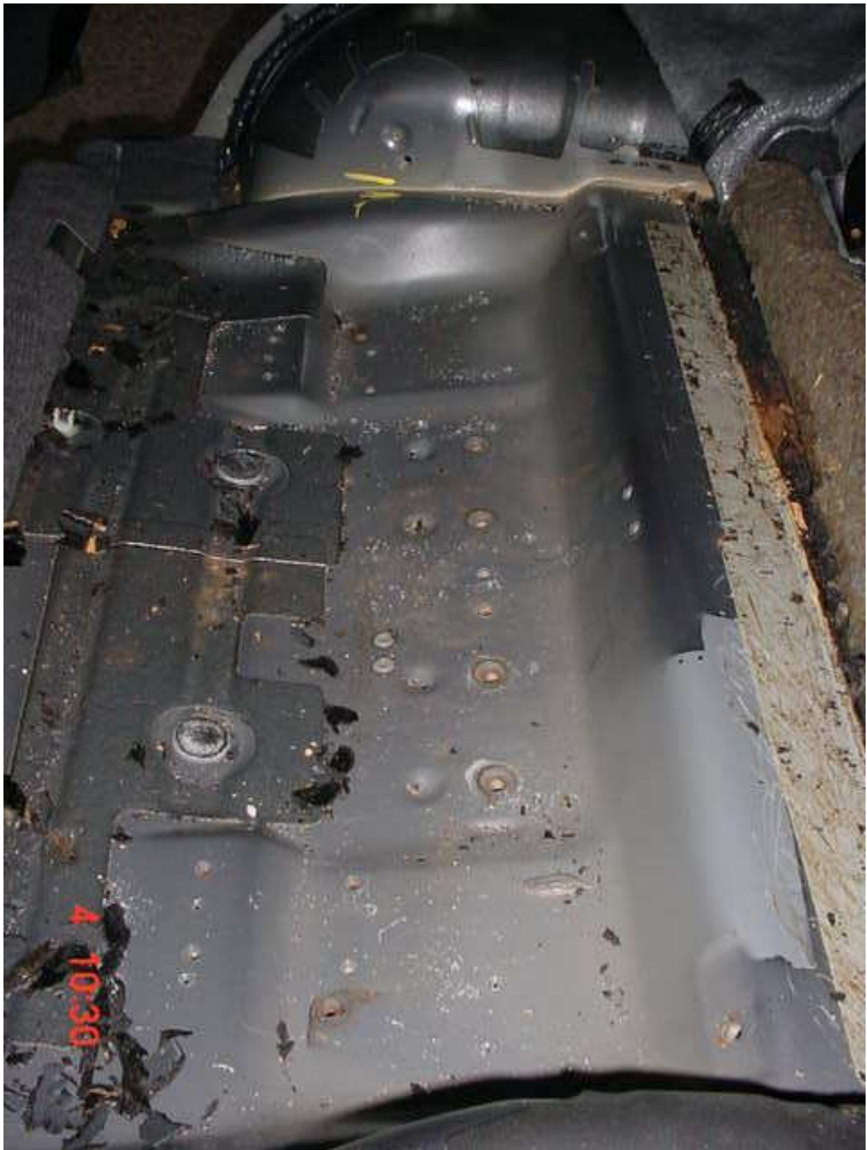
Terrano floor, inside vehicle, with seat removed, photo taken from left rear door opening, very little visible rust was showing in the interior of this vehicle.
