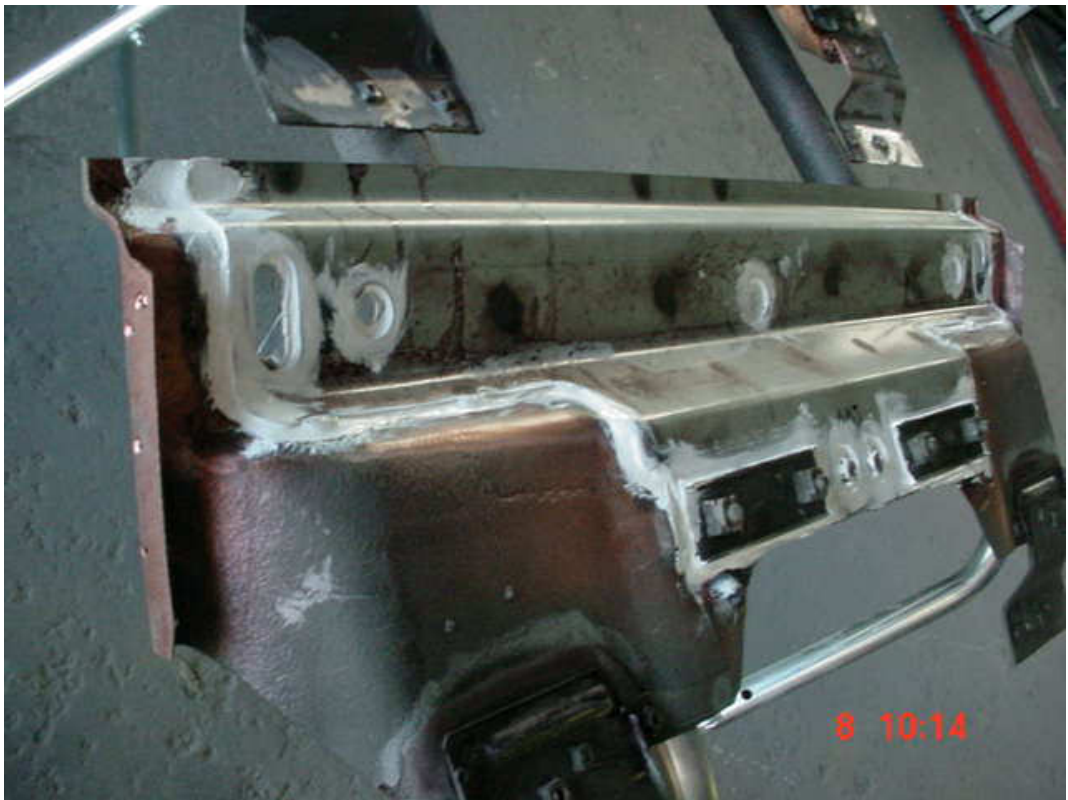
Urethane sealant has been applied to all edges of the LVV load-bar where it mates with the reinforcing plate, to provide a complete seal.
