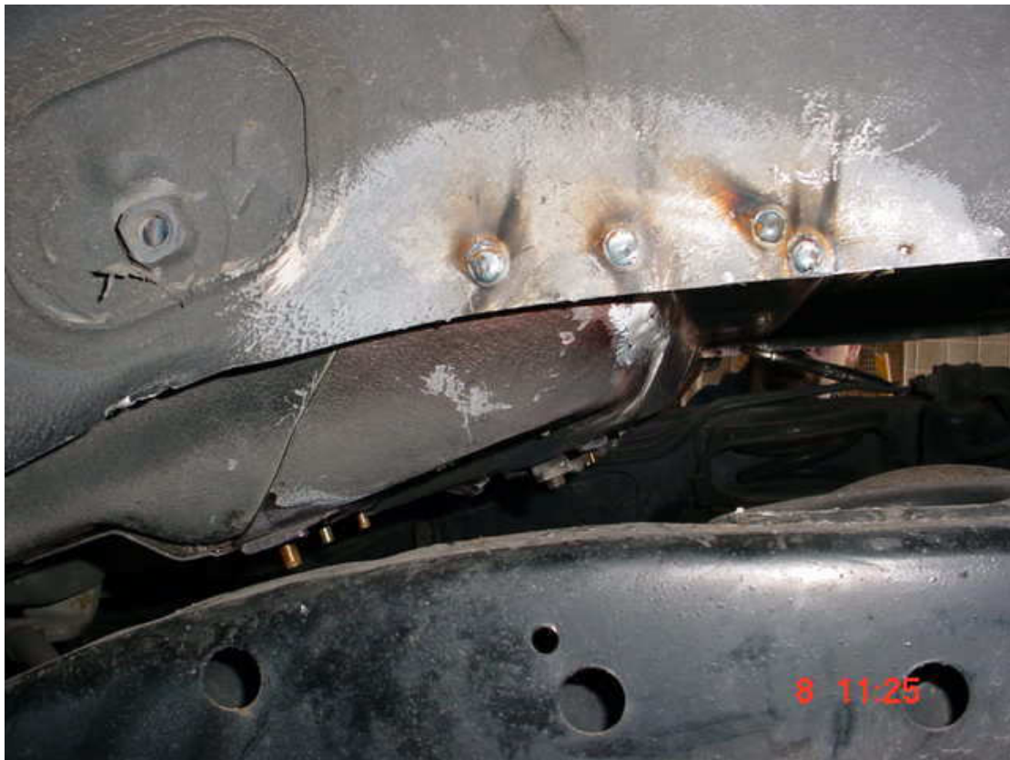
Plug-welds in wheel-arch area have been completed, ready to grind flush.
