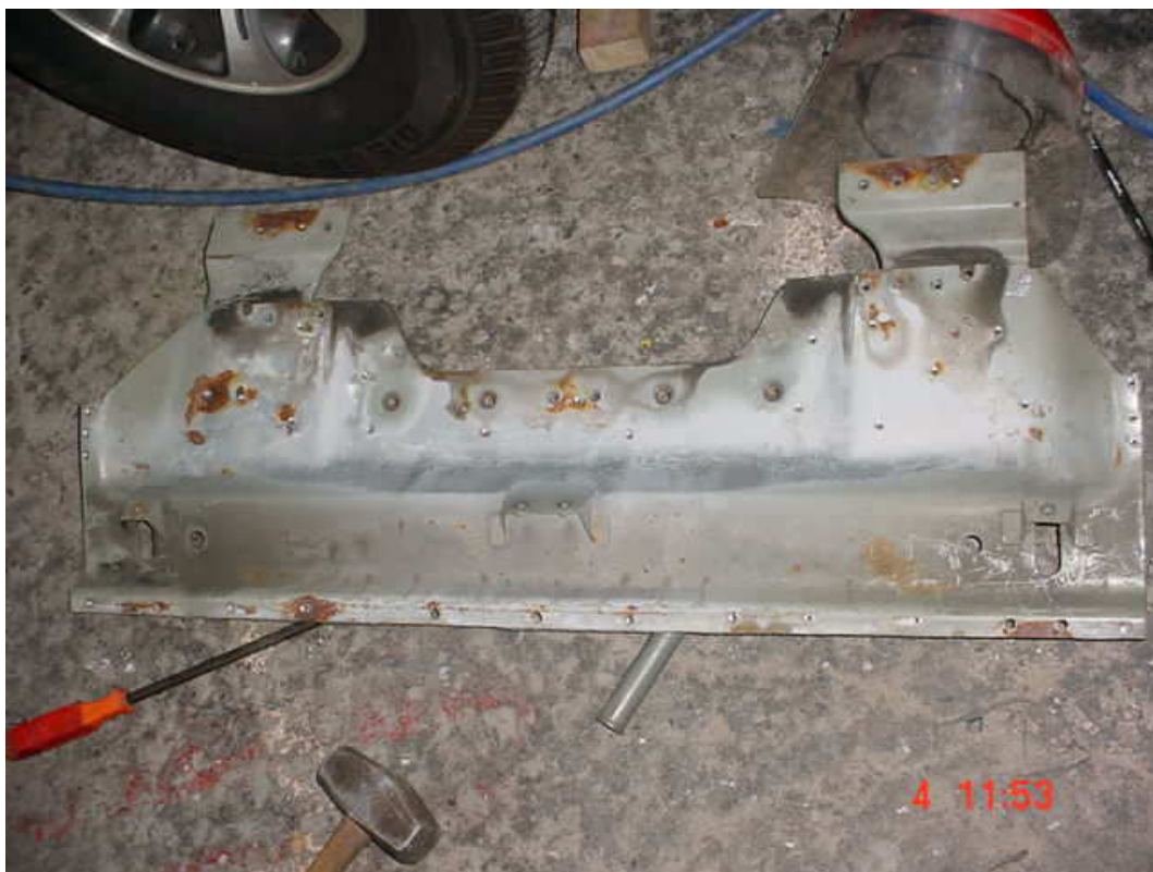
The reinforcing plate upper face (hidden from view when in the vehicle) is inspected. This example is one of the better ones. Any patch repairs to the reinforcing plate are done at this stage.
