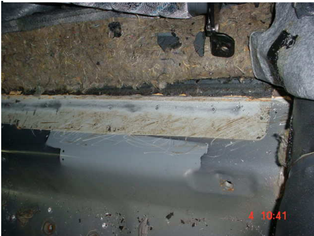
Interior of vehicle floor, spot-welds have been drilled through using a 2mm drill bit, through both the central floor section and the reinforcing plate (2 layers).
