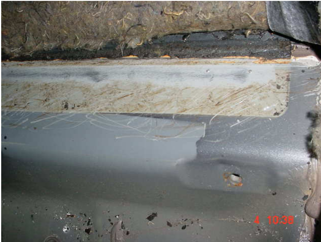
Interior of vehicle floor, stripped back to bare steel with wire wheel to reveal spot-welds.
