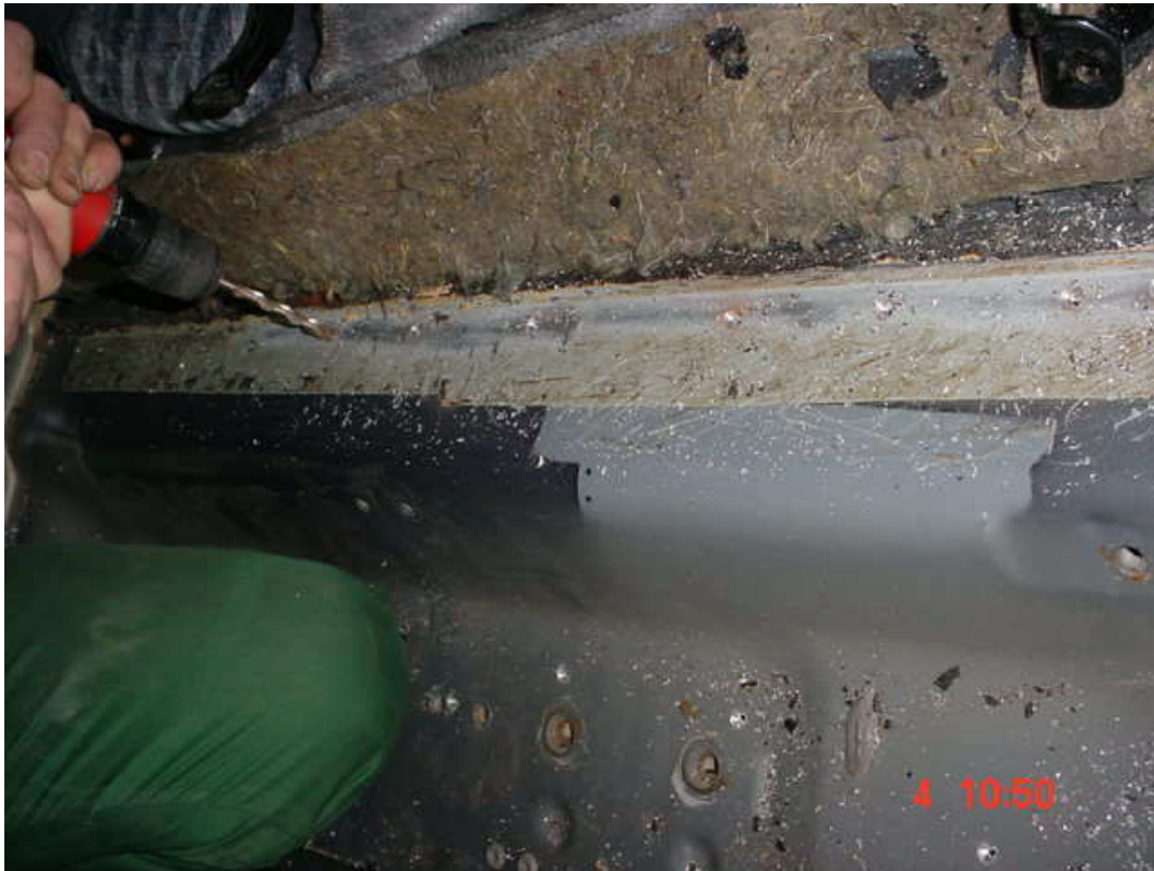
Interior of vehicle floor, spot-welds drilled 8.5 mm through the central floor section only, (1 layer), ready for later plug-welding.
