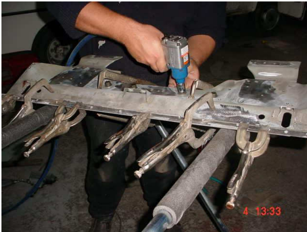
Seatbelt bolts through the seatbelt-anchorage plates help clamp the assembly for welding.
