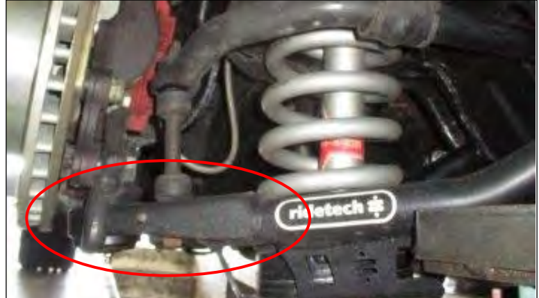
Image 2: This is an example of a Ridetech Chevrolet C10 truck lower arm with cantilever-style ball joint design.
