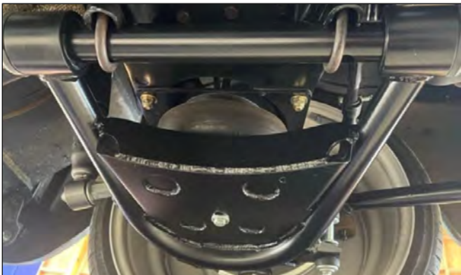
Image 8 and 9: This is the Ridetech lower control arm shown in Image 7 after significant rectification work to reinforce the ball joint bracket, and eliminate the sagging in the air bag mounting plate. LVVTA thanks Custom Street Rides (CSR) for their assistance with developing and testing this rectification.
