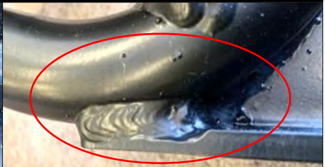
Image 6: This is an example of a weld at the ball joint end housing (a highly loaded part of the arm) which has significant undercut, a weld defect that reduces the thickness and strength of the parent material.
