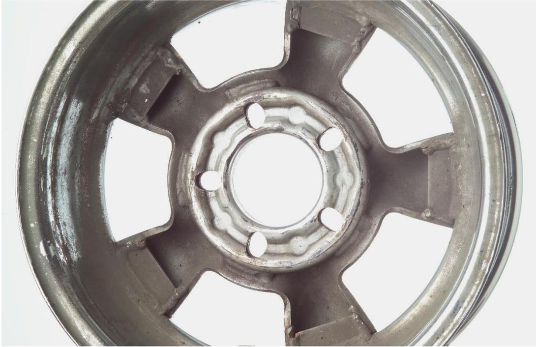
*View of back-face of poorly designed and assembled 'Supreme' wheel.*
