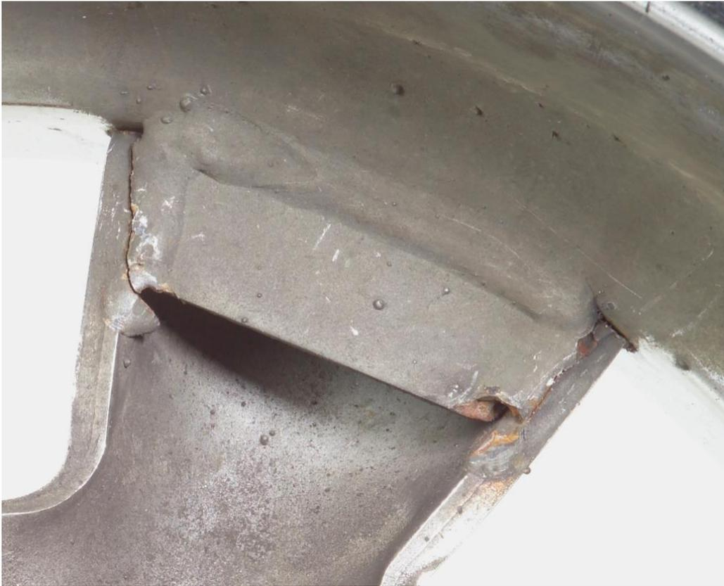
*Closer view still, of weld failures.*
