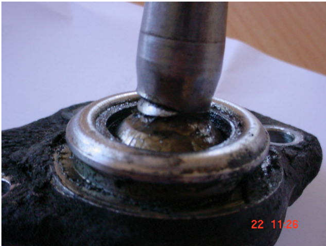
The deep groove in the 'Camelot' brand balljoint shaft has been caused by the high loads.
